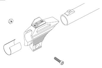
On barrels with a bead base, first remove the bead by unthreading it with pliers or other appropriate tool.
