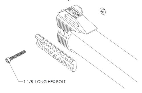
The rail fits on both versions of the Front Sight (with or without magazine extension tube) and locks in place with a unique taper fit. It is strongly recommended to not mount anything that extends past the shotgun barrel.
